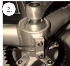
The drawback to these types of eccentrics is that the threads on the frame can strip out, or the brazed-on threaded piece may even break off of the frame entirely. This requires a costly frame repair and paint work. The sharpened bolt style also has a gouging effect on the aluminum chunk (kind of crude we always thought).
