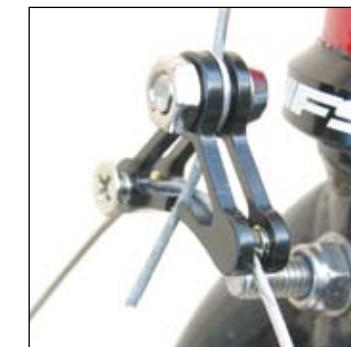
Getting the straddle cable length right was a job requiring three hands, and reference to the pictures on R&E's website to get the angles about right. A detailed video instruction set is apparently in the works. But it wasn't hard, really, just a bit of trial and error.
